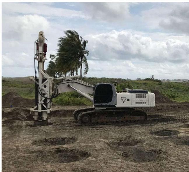
Figure 1. RIC attachment mounted on excavator
